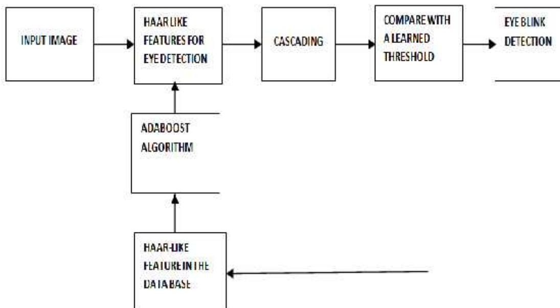
**Fig. 2: Illustrates the Various Functional Stages for detecting the Eye Blink**
